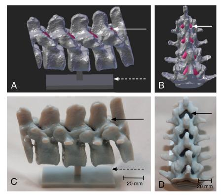
FIGURE 1. Digital model of the printed phantom, as visualized from the side (A) and from above (B). This model comprised osseous structures (gray), the ligamentum flavum (solid arrow), and the pedestal (dashed arrow). In the corresponding printed model (C, D), the osseous structures and the stand (dashed arrow) were gray; the ligamentum flavum (solid arrow) was black.
